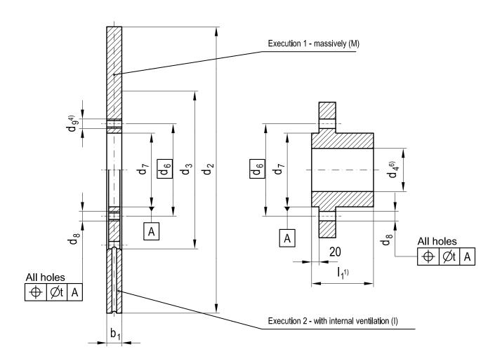
Disk brake with hub acc. to DIN 15 431
